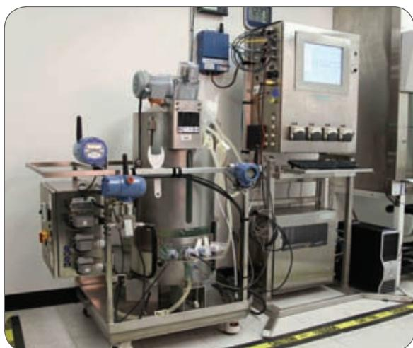
Figure 1. Single-use bioreactor with wireless transmitters and a lab-optimized DCS.
