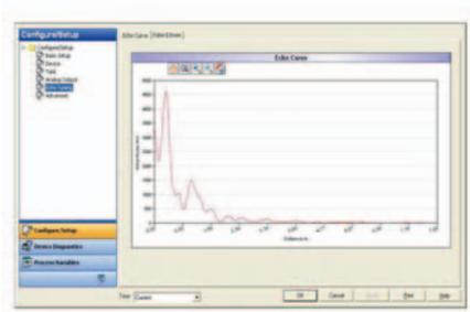
A radar level gauge with two different hosts. The same information has a different 'look and feel.' The device determines what will be displayed, while the host control system determines how it will look. This ensures all displays on a given process control system have the same look and feel, regardless of the device supplier.
