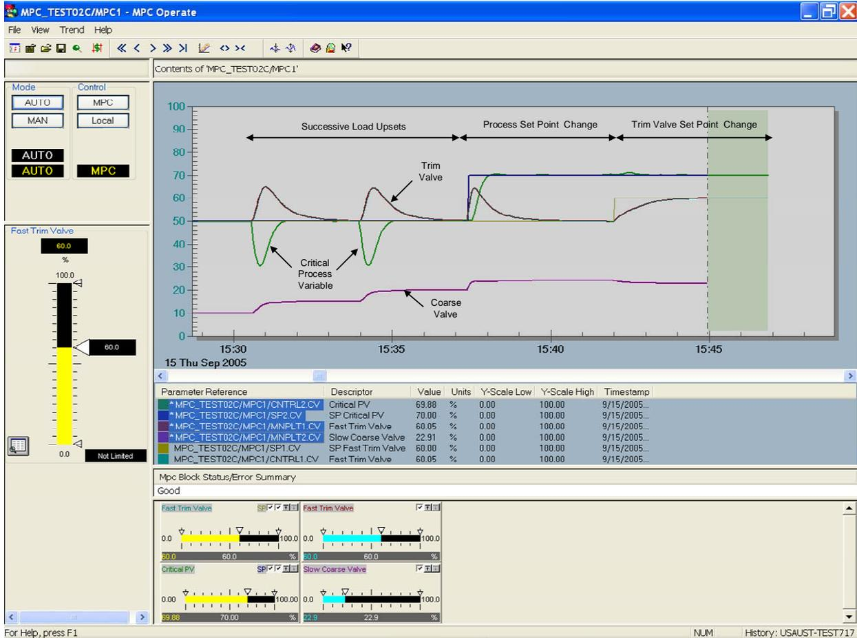
Figure 5-1b Trend in MPC Operate of Response of DeltaV Predict to Disturbances and Set Points
