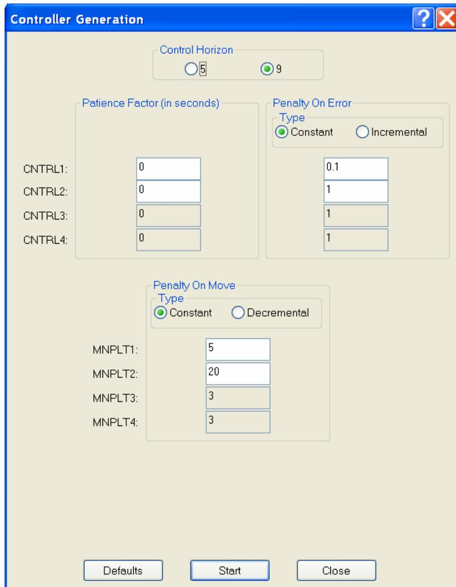
Figure 5-1a. Penalty on Moves and Errors on Controller Generation Screen in DeltaV Predict
