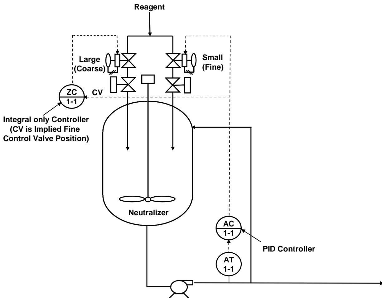
Figure 2-1b Valve Position Controller for a Neutralizer
