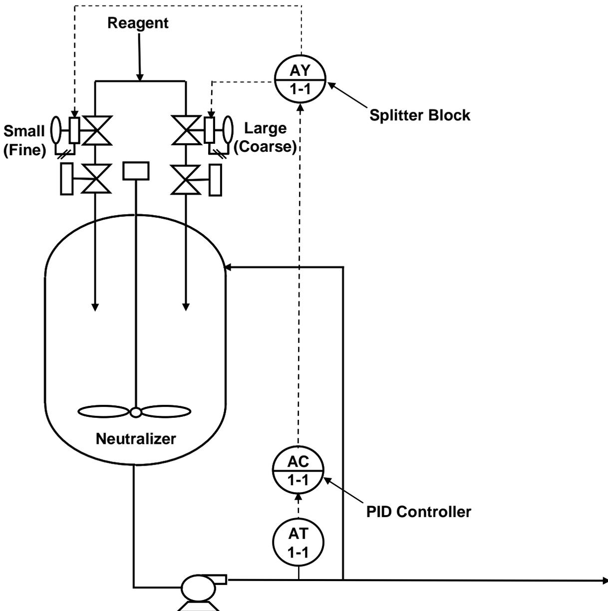
Figure 2-1a Split Range Control for a Neutralizer
